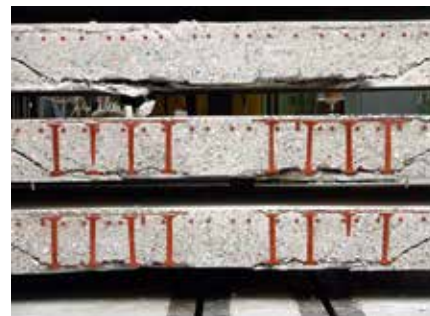
ancoPLUS®-Zulassungsversuche ancoPLUS® - approval tests
